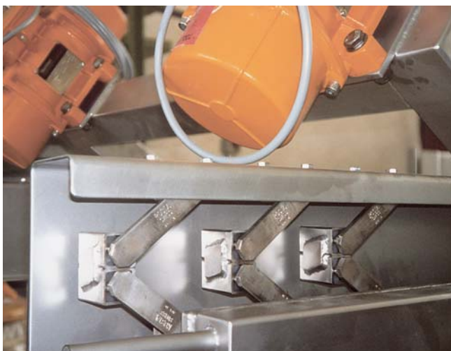
Stainless steel AB's supporting salad feeder
