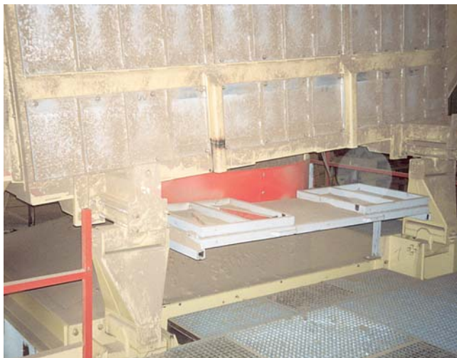
Support of heavy gyratory sifter with AK
